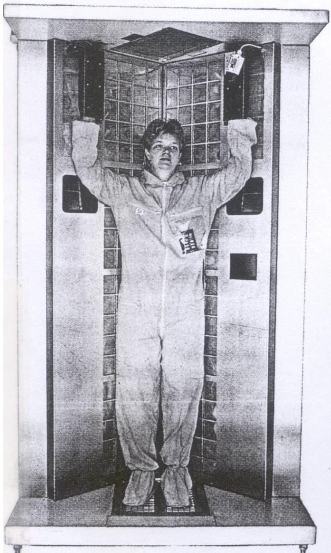
進出輻射管制區之門型偵檢器 The Gate Detector installed at a gate of a radiation control area
