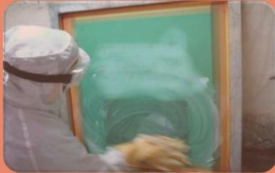
Cleaning the ink residues on the screen printing template is a manual task in this PCB manufacturer.
